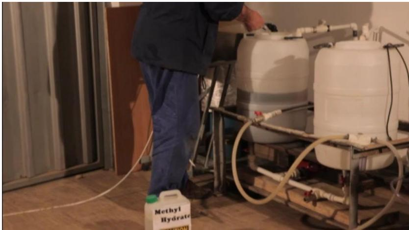
After this is done, we transfer the mixture from one barrel to another, several times, checking the temperature in the process.
