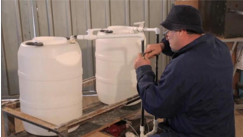
I'm using the PVC tape because it makes the connection with the taps more much easier to do.
