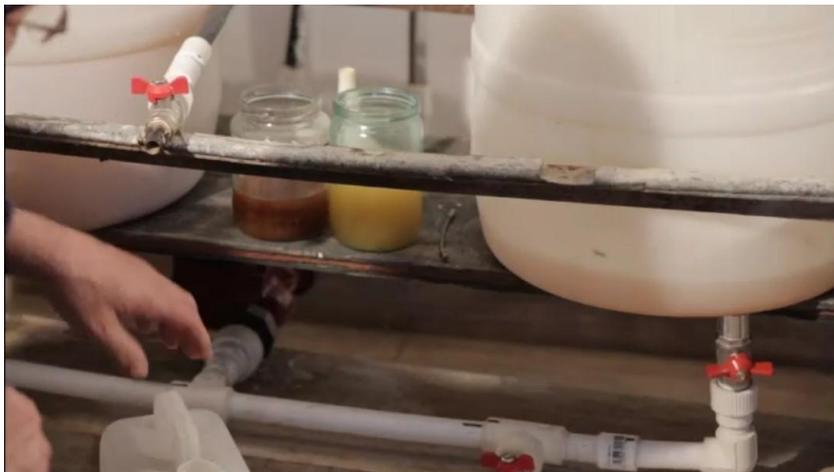
We transfer the mixture from the first barrel to the second, then we are going to raise the temperature inside the barrel with a heating coil.
