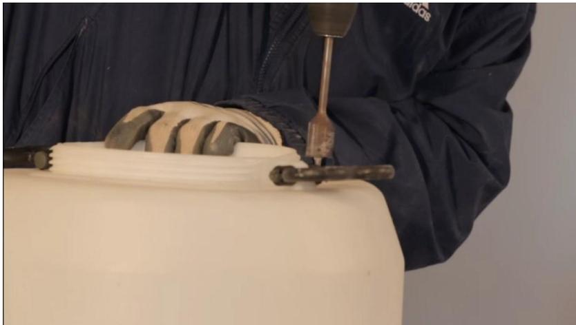
I will use a steel ribbon with some self-drilling-screws to hold in place the pipes.
