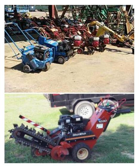
We selected a Ditch Witch which was probably second choice, but it did have the advantage of being 'maneuverable'. It turns out that this type of machine has no real steering, it just goes backwards in a generally straight line and digs as it goes. Changing direction is not easy and consists of grabbing this horribly heavy machine and using all of your strength and moving it a few degrees, then repeat until properly positioned.
