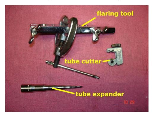
So, in addition to the tools previously pictured, here are the tools I'll be using:
