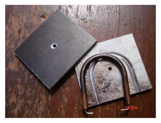
This shows the plates milled out to accomodate the heater element. I also milled a plate on my drillpress using a quarter inch drill-bit. It looked like hell but worked. Howard has a NC shop and did a perfect job in just a few minutes (shown). Not shown in this pic is a channel I drilled out to recieve the temperature controller probe.
