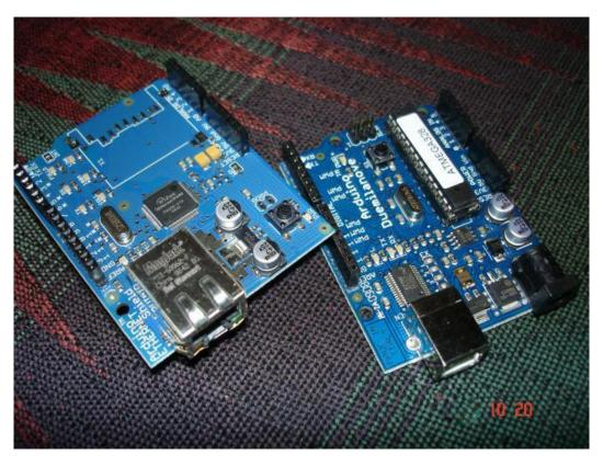
I got both of these boards from Spark Fun. The on on the left is the Ethernet Shield and the one on the right is the Arduino board.
