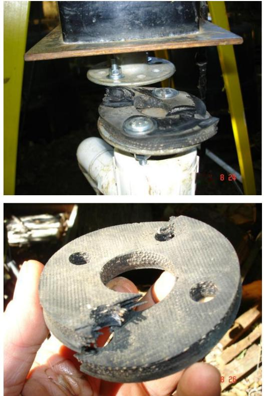
So my solution was to use stainless bolts to bolt straight through the doughnut and add some rubber washers atop the flanges capped with big washers, and adjust the nyloc-nuts to 'barely snug'. Under off-
