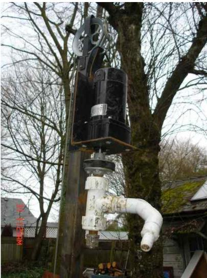
This is the gear motor head. I fabbed an 'L' bracket for the motor and used a 2" square tube for the vertical, and a close-fitting 2" inside receiver tube welded to the L bracket. it slides up & down well and doesn't have too much slop. You can see the hand cranked wench to raise and lower the gearmotor head. It's not optimum, but it works OK.
