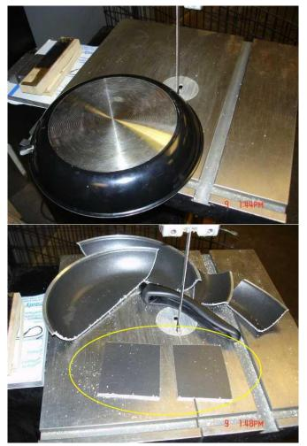
This will give me non-stick surfaces for fusing the poly pipe.
