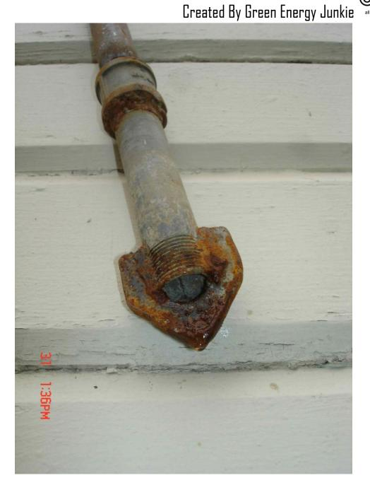
This is a detail of the business end of the auger. The water gushes through the pipe and flushes out the drill-cuttings. I have come to understand that the water is definitely part of the tool. It contributes more to the advancement of the drill than any effort on my part.
