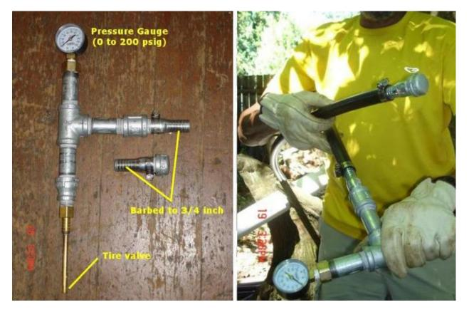
Here is the pressure tester I made up for the job:
