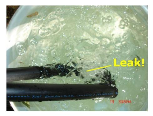
There was nothing subtle about the leakers, they were very easy to spot with the air-pressure/water test.
