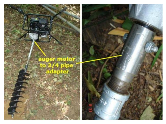
To my disappointment, the post hole digger didn't exhibit the advantage of power I had expected. I tried putting water in the hole a couple of days before drilling, but when I hit the tough layer of clay, it wasn't just tough but it was tough and slippery.
