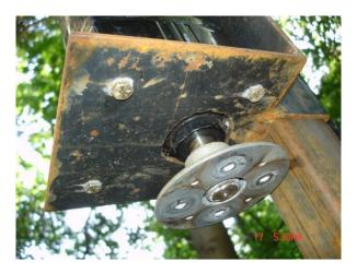
Here are the vibration dampers I use to tie the two flanges together. I use nyloc nuts to prevent them from backing off during use. Works great.
