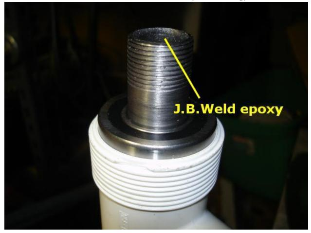
I stuck some bread dough about an inch down into the top end pipe and filled it up with J.B. Weld to form a plug so the water wouldn't get out.
