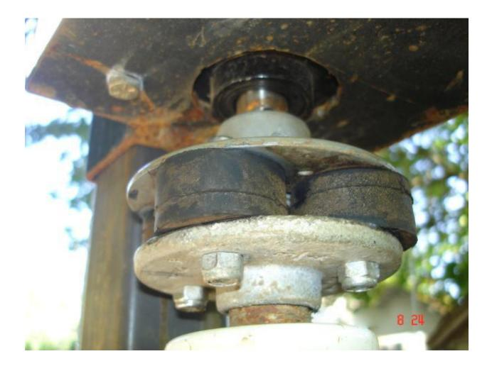
My flexi-joint on the electric auger was not holding up so well to all the punishment I have been putting it to.
