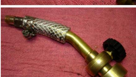
First I unscrewed the flame tip from the propane torch, which was worthless for brazing anyway.
