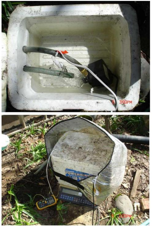
this shows the set-up in the cooler box. I initially thought that it would be a good idea to put the coffee cup warmer inside of something so it wouldn't melt the foam box. I nixed this idea, and suspended the heater from the hose with a bread wrapper twist-tie.
