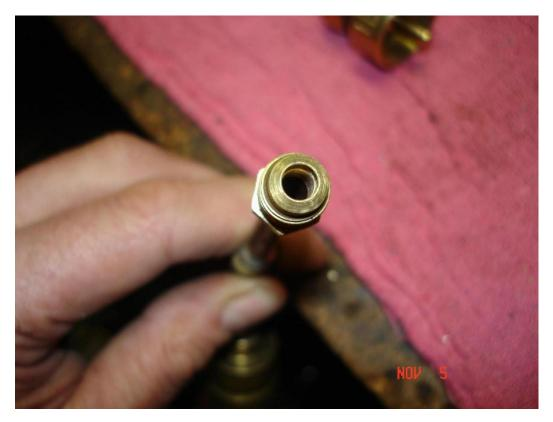
I didn't put the Schrader core back into the valve, because with the needle valve of the torch, there's not much need.
