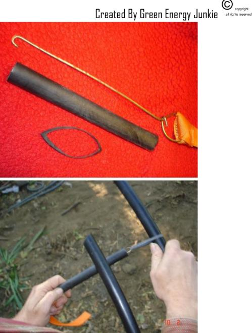
As shown in the bottom pic, the rubber band would be slipped over one leg of the loop, then the wire hook would be pushed through the spacer tube, hooking the rubber band. Then the hooked rubber band end would be pulled through the tube and slipped over the remaining leg of the loop. Several of these would be put over the loop, then slid into place at desired intervals.
