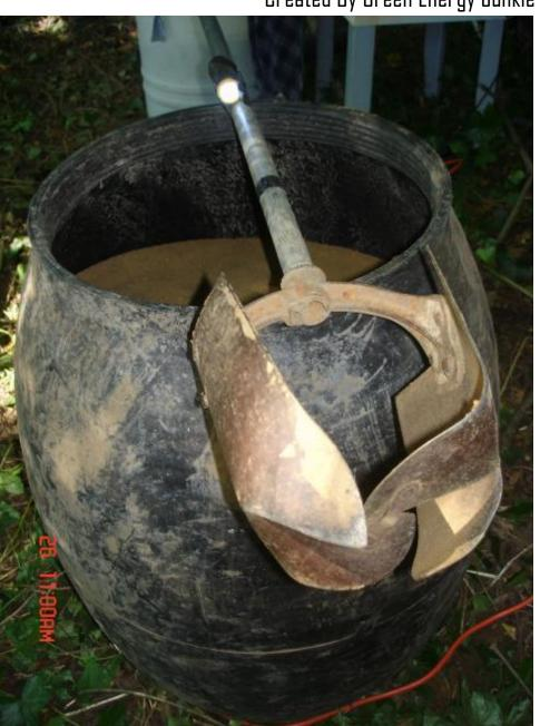
I make a temporary mark on the electric auger's vertical tube to keep track of drilling progress and let the auger do the work. I have found that after it has dug about 4 inches, the auger bucket is full, so I use the shop vac down the hole to vacuum out the debris and then drill down another 4 inches, etc.
