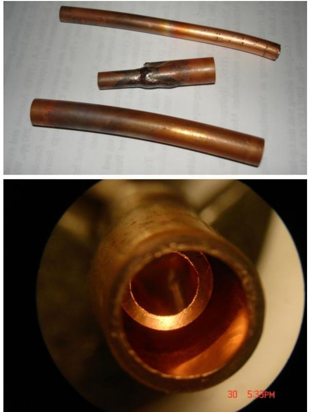
Bottom photo tells why... This is a microscope shot down the barrel of the tube I just brazed. The cut was made about 3/4 inch from the brazed joint and about 5 minutes earlier, it was glowing cherry red. As you can see, there is no copper oxide, not even any discoloration.
