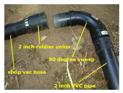
I use the hose clamp on the shop vac side, and use the rubber side loose on the PVC side. When the shop vac is running, the suction keeps it all together very well. The surprise benefit is that the 90 degree bend gives me a handle for rotating the pipe. And best of all, no more vacuum-hose kinks.
