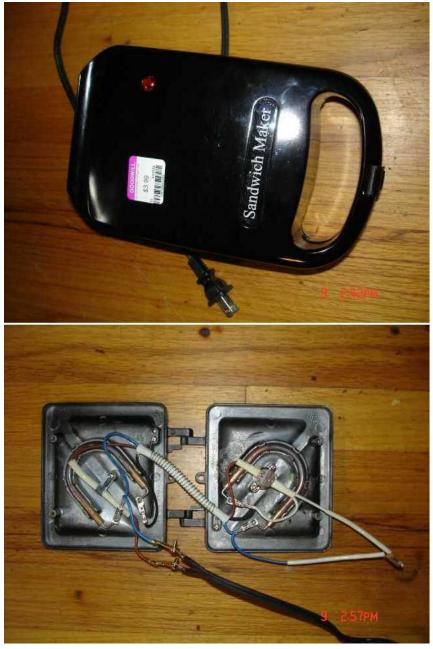
This device drew 600 watts, which I properly guessed ran 300 watts per side:
