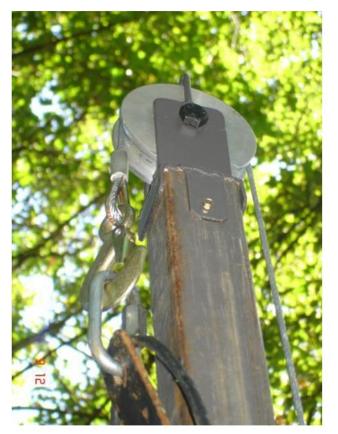
So I bought a winch-grade pully and rebuilt the pully-carrier, this time with much stouter steel.
