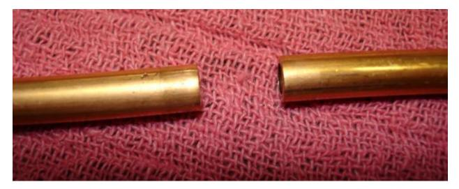
Since refrigeration is subjected to vibration, a butt joint will not do, so the trick is to expand one piece of tube so that the other tube will fit inside.
