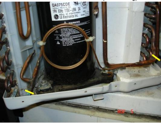
This tiny coil is called the 'cap tube', no relation to the capacitor...
