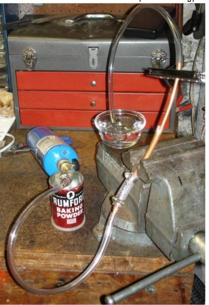
The gas from the propane bottle feeds into the tubing, via adapters to the tube to be brazed. The vice acts as a heat sink, but not very well. I may get another cheap flaring tool to use as a heat sink because the one I have over the brazed part is working very well. More surface area around the tube to carry off the heat. Finally, the tube from the other end of the brazed part goes into a dish of water, to act as a flame trap and also as a visual indicator of the volume of gas that is flowing.
