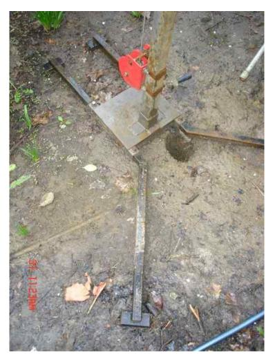
This is the base of the gearmotor auger I put together. Based on my hand-drilling experience, I figured a small motor would do the job, so I got a 1/4 HP 25:1 permanent magnet gearmotor off ebay for \$70. A 1/4 HP motor doesn't require a huge amount of structure to support and control, so fabrication was pretty easy.
