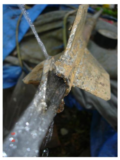
As you can imagine from a dirt's eye view, with this thing coming at you, rotating away, and water blasting out all the clay and sand debris, the clay just doesn't stand a ghost of a chance.
