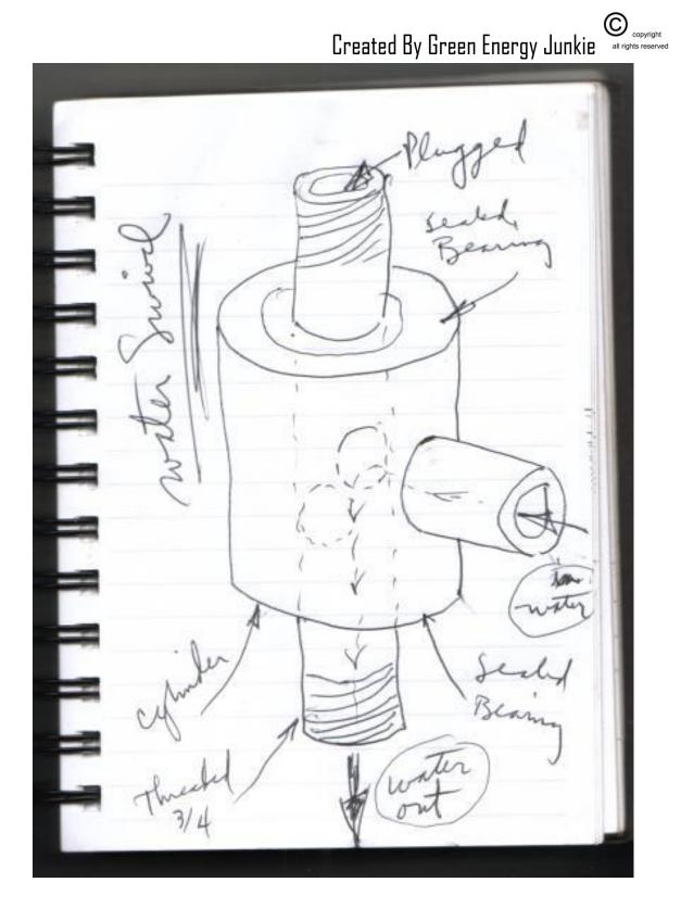
I forgot to label the holes that are drilled in staggered positions (for strength) on opposite sides of the pipe.
