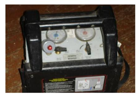
Basically, they are both turned to the "Self Evac" position and the unit is run until a full vacuum is pulled, as shown in the top photo below.
