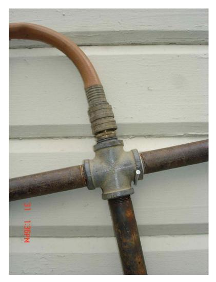
This is a detail of the swivel end of the auger. The swivel adapter is not exactly the same as 3/4 pipe thread, but by loading lots of teflon tape onto the threads, I got a satisfactory seal.
