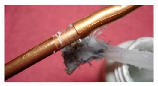
Here I'm applying silver-brazing flux to the tube that will slip inside.
