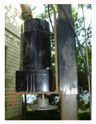
I welded the motor bracket out of 3/16 steel. It could use some reinforcement at the corner.
