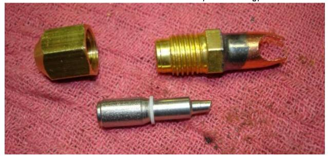
This valve has a removable core, with a tiny plastic gasket, and a brass screw-on cap. The core must be removed, then the piercing valve body is brazed into place on the still-pressurized refrigerant line, then the core is inserted and the cap is screwed down tight, driving the point of the core through the refrigerant tubing.
