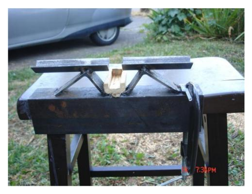
I did improve this jig from previous photos by using a wooden rest for the heater. this rest perfectly centered to heater on the pipe.
