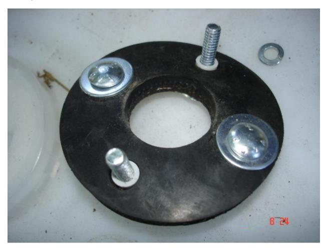
So I tried a Ford/GM steering doughnut replacement part, set up the way it was designed and it worked just fine for about three glorious, high-stress minutes before failing.
