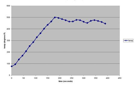
This is a graph of the unit heating up when the dial is set to "400".
